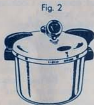
Turn cover counter clockwise until cover hits stop and arrow points to "open" as in Fig. 2.
