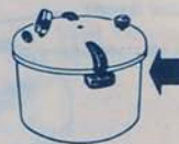
Cover handles are directly above and between lines of Cooker handles, as in Fig. 6.
